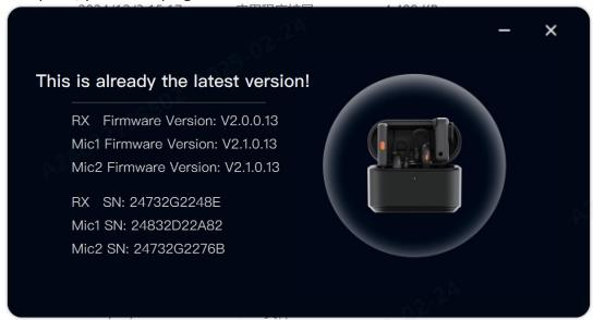
6, If the upgrade fails, follow the prompts to disconnect the connection between the RX and the computer. Wait for the device indicator light to change from magenta back to green/blue and remain on, and then reconnect for upgrade.
