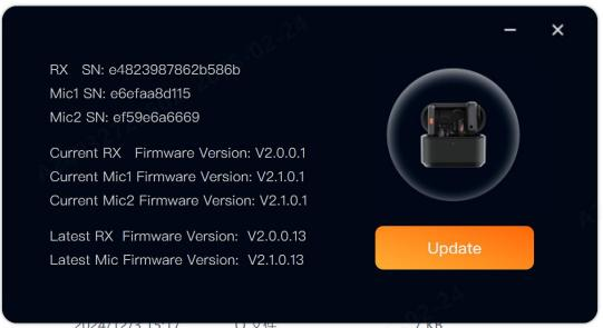
4. Click "Upgrade TX, RX" to enter the upgrade state. The upgrade process takes about a few minutes. During the upgrade, the TX and RX indicator lights will be magenta and remain on. When the upgrade progress bar on the host computer is completed and the upgrade success interface is displayed, it means that the microphone upgrade operation is completed.
