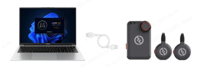
3, After the TX and RX are connected to the computer, the host computer will automatically identify the device and obtain the latest firmware version information. (If the information acquisition fails, click "Retry" to obtain it again).
