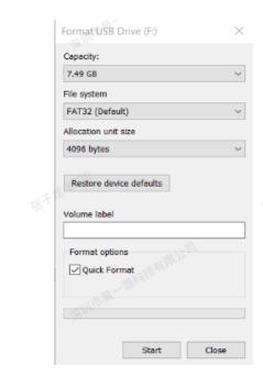
2. Insert the USB flash disk into the wireless monitor's Type-C port will the monitor enter the updating status automatically after 1 mins around. Then just waiting for the updating completion.
