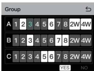
5.4 Default grouping: All the beltpacks and the 2-wire and 4-wire audio systems are in group A. In this case, the group A indicator light on the beltpacks will turn on.
